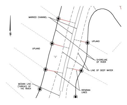
For example, at area "2" above, perpendiculars are constructed at the nearest channel edge and run back to shore.
