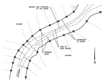
For example, at area "1", the red riparian line is the "docking" line shown perpendicular with the dotted median line stopping at the line of deep water. The dashed extension of the riparian line is the "view" line out to the median line. These lines are: not on the extension of the upland side line, not perpendicular with the water boundary, or not perpendicular with the line of deep water.
