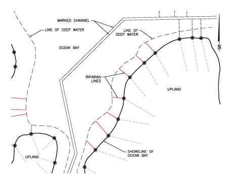
**Inlet Channel – Perpendicular with Channel Line** At the inlet of the ocean bay, the proximity of the channel is now the important consideration, and perpendiculars would be dropped from it as shown.
